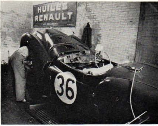
Some last minute adjustments at Le Mans, 1950. The racing dash is very neat, a steering-column shift unusual on a competition car. Jowetts were one of the first production cars to have a fully opening front. (Photo: Mr. Louis Klemantaski)
