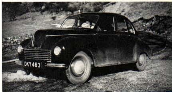
Much testing took place on Yorkshire test hills, including Sutton Bank. This is the second prototype with its designer at the wheel; it will be noted that the four doors are no longer interchangeable (as they had been on the first prototype) but all panels are very flat, for fabrication by simple methods. Bonnet and grille were changed before the car went into production, and at this stage a flat two-piece Vee windscreen was used.
